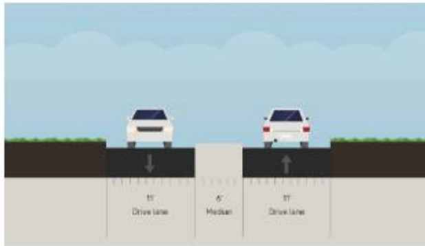
MEDIAN TYPICAL SECTION
